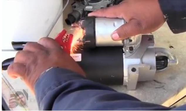
The motor should spin but the override clutch should not engage, i.e. slide forward.
