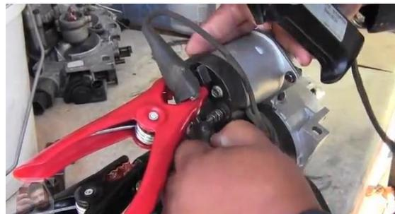
The override clutch with the gear should slide forward to engage the flywheel and the starter motor should turn. If it does not, then the solenoid needs to be replaced.
