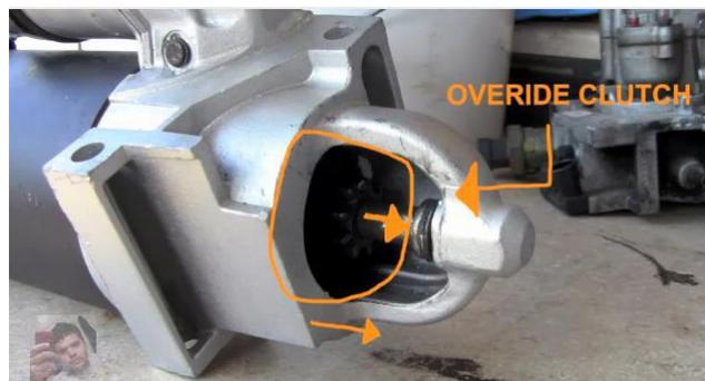
**Testing the Motor Only:** The motor is what gives the flywheel torque that is needed to start the engine. Leave the battery negative cable connected to the starter housing and touch the positive cable to the motor terminal identified in the picture above.
