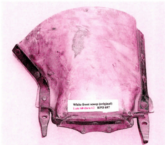
Front Air Intake Duct from RPO 687
