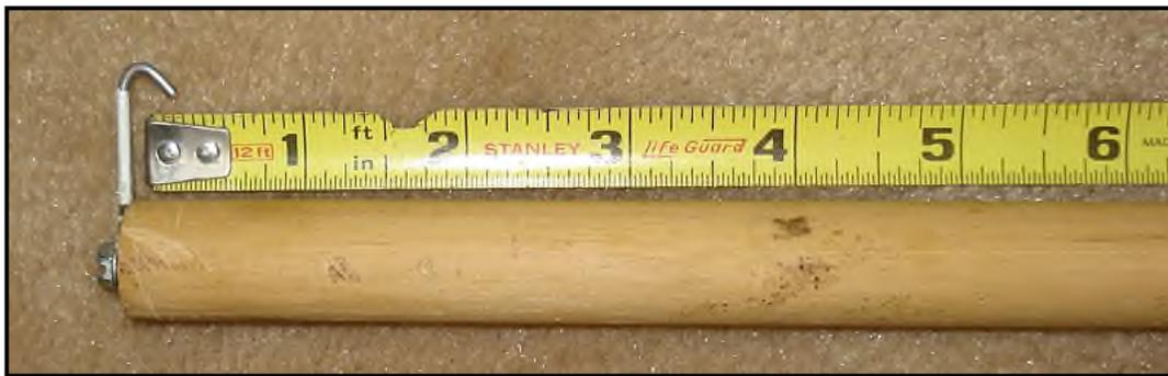
I bent a piece of coat hanger to make a loop to screw to the top of the dowel. The hook portion is about 1" (13/16" actual). You will need the hook to catch the spring lever on the latch
