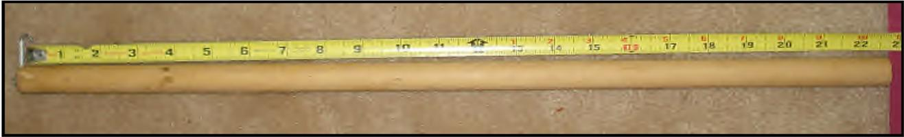
$\frac{3}{4}$ " dowel with hook on the end. This piece is 22.5" long and it just rests on the large splash shield of my '65 AC coupe down under the AC box.
