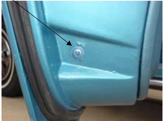
Figure 8: Rear channel mounting screws. These retain the rear window channel (see Fig. 7) to the back of the door.
