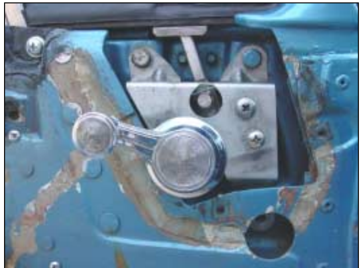
Vent-window regulator installed in door
