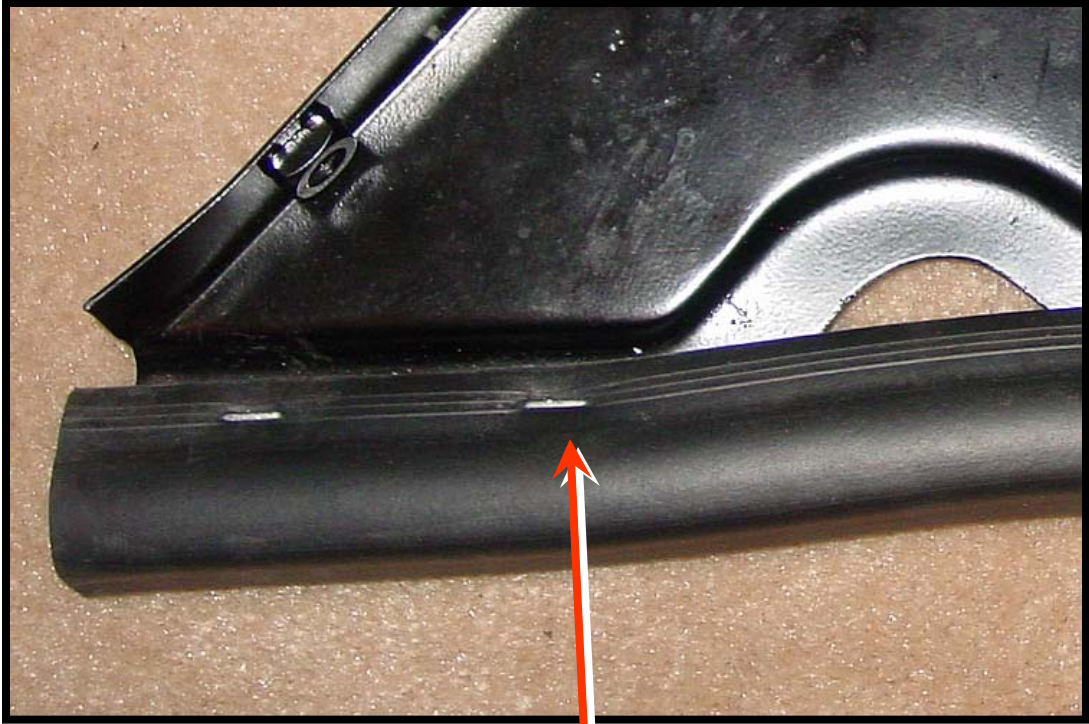
Finished staples top and bottom
