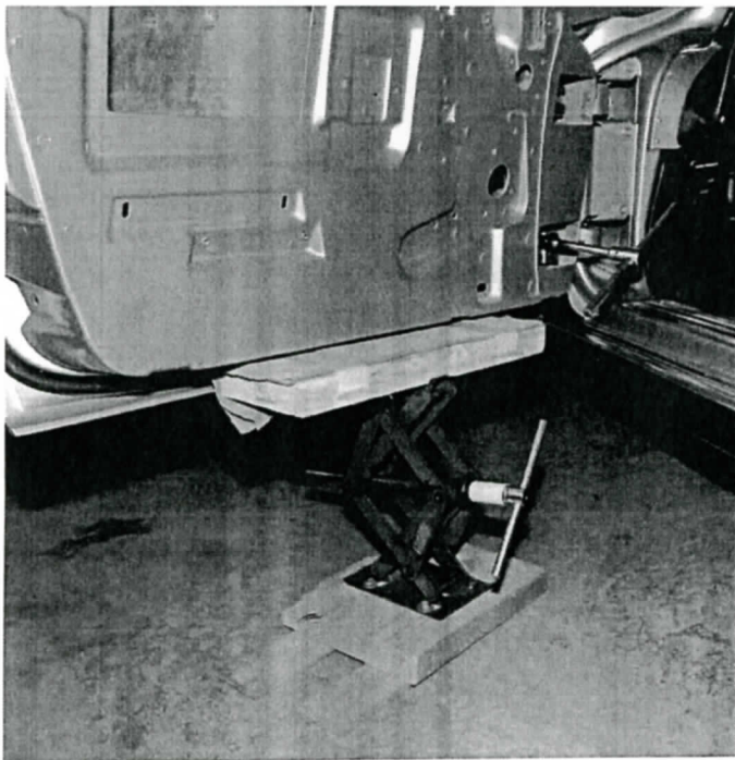
Door jack in use. Note construction shims used for leveling.
