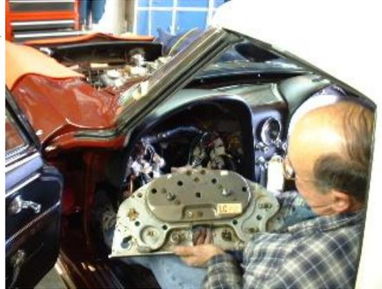
This is a **BIG TIP**--- prepare paper dots ahead and tag as you remove --- Send the cluster out, or if only one gauge needs service such as the speedometer you can of course opt to send out only the piece --- the best bang for your buck for the cluster seems to be auto instruments.com --- they will rebuild the tach and speedometer and recalibrate small instruments for \$140 (this includes return shipping)
