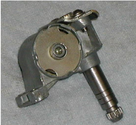
The problems I found are as follows: The grease was hard and gummy. The housing was slightly deformed evident by the bore where the sector gear plate fits not being round. The worm drive retaining plate was loose on the rivets creating excessive backlash. The sector gear had the last 2 teeth worn and deformed. No problem. We can fix this stuff.
