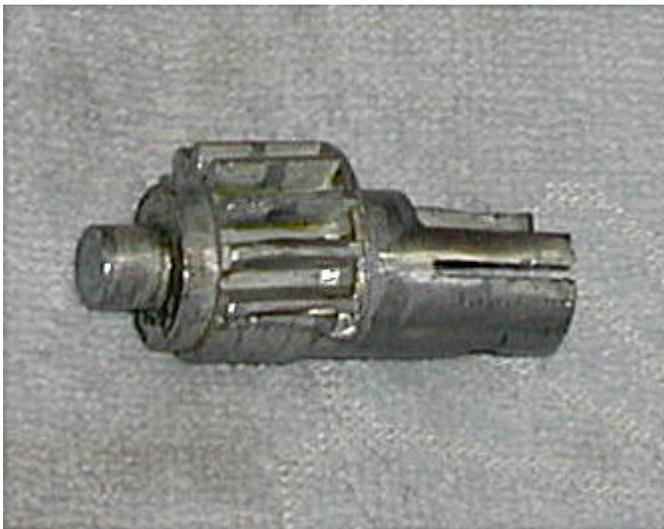
Now for assembly: Grease all gear teeth and bearing surfaces with lithium. Install sector gear, thrust washers and spring washers. Squeeze the assembly together lightly using 2 sockets in vise (just enough to compress the wave washer) and stake over the housing lip in 4 places with
