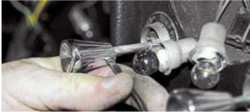
Old school knob removal requires a small flathead screwdriver to loosen the set screw. Once the set screw has been loosened, turn the knob counterclockwise to unscrew. Most of the knobs have these set screws at the bottom of the knob when the switch is turned off. If there is no screw present the knob twists off counterclockwise.
