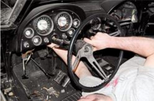
First, remove a couple of Phillips head screws holding the column trim, and take off four 1/2-inch hex bolts and nuts. Then the column comes out. I did go out under the hood first and remove the 7/16-inch 12-point bolt holding the steering coupler to the steering shaft. This gives me plenty of room to work in the interior.
