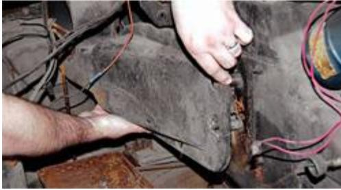
You need to drain the cooling system at the radiator and then go under the hood to remove the heater core. Next, carefully remove the heater hoses to avoid heater core damage. I usually slice the hoses along the heater core tube and peel it away. You should never tug on any heater hose at the core to remove it. Once the hoses are taken off, remove the 7/16-inch hex nuts from around the perimeter of the outside plenum cover.
