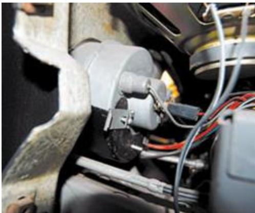
Clocks are held in place with these retaining clips that require a downward push near the retainer stud. Pull outward on the retainer clip while pushing downward. The electrical connectors and lamps can be removed once the clock has been removed from the dash.
