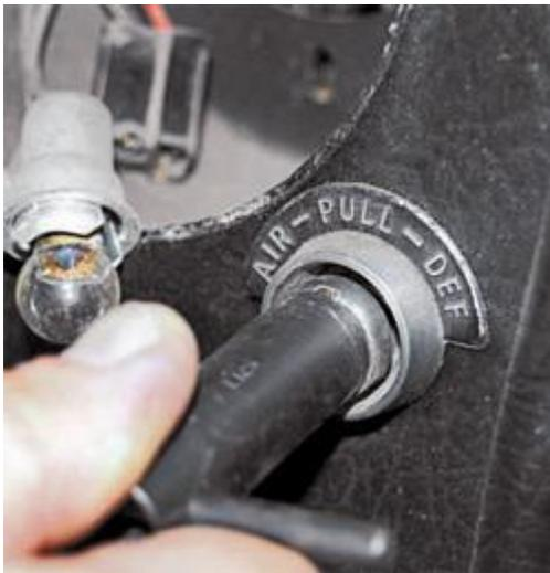
This Corvette Central special tool (PN 251004) makes removing and tightening the special cable retaining nuts easy, and it works on the headlight and wiper switches. Two ignition-switch nut wrenches are available (PN 251003 for 1960 to 1965 Corvettes and PN 252001 for 1966-1967 Corvettes). I see ignition switch bezel nuts scarred up all the time from "Mr Goodpliers" at work.
