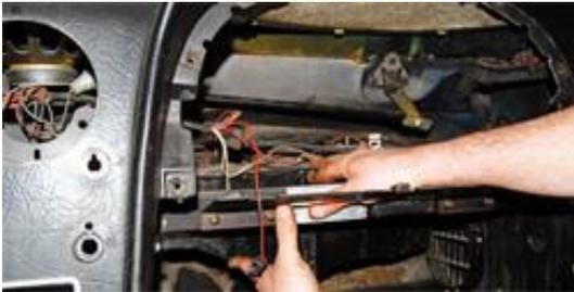
needle-nose pliers to grasp the clip and wiggle it upward. With careful removal the clips can be used again.
