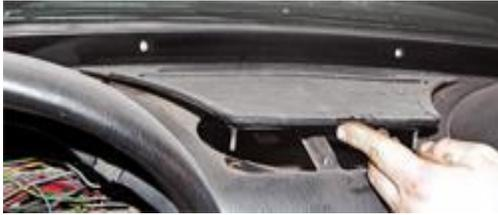
The reason to make a big deal about this grille is late-model dashes have plastic speaker grilles snapped in place. Prying this fragile metal grille up distorts it. If you do this, you have a difficult time making it lay flat against the dash. The speaker grille frame is made from pot-metal, meaning they break if you try to modify their shape. There is some shaping (very little, though) or snap.
