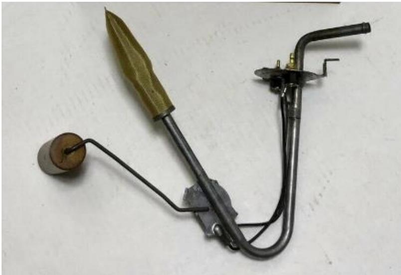
Conclusion: the repo sending unit outlet tube is bent at an incorrect angle, allowing the car to "run out of gas " with 2 to 3 goal of gas remaining in the tank. and looking back on my installation of the repo sending unit a month ago, I seem to recall that inserting it into the mounted tank wasn't as easy as installing an OEM sending unit. Fortunately, I was able to locate an OEM version and replaced the reproduction version.
