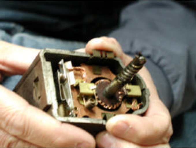
Remove the brush assembly by pressing up on the retaining clips as shown. Remember the one against the curved side is soldered to the housing.
