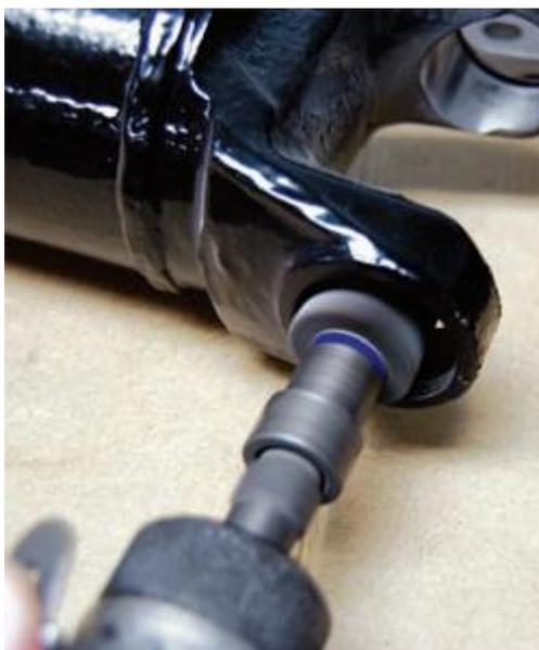
Once the driveshaft or axle shaft has been disassembled and cleaned, use a 3/4-inch-diameter flap wheel to remove any remaining corrosion. Tread lightly here because it is easy to remove too much material and have loose-fitting universal joint cups.
