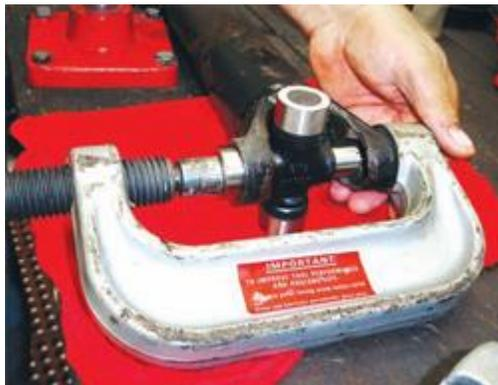
This is the preferred method of universal joint replacement. This massive OTC tools C-clamp has multiple uses, and here it pushes the U-joints out effortlessly. The C-clamp also makes easy work of installing the new U-joint cups.
