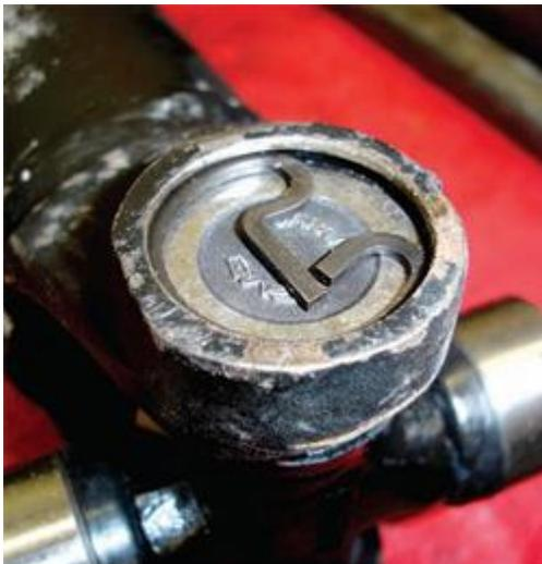
Make sure that the U-joint retaining clips are fully seated in the groove. If the retaining clip comes out of the flange, the U-joint cup follows. It does not matter how tight the cup fits in the flange.
