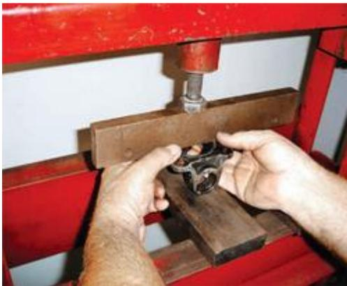
Careful work at the hydraulic press can straighten the flanges for reuse. The trick is to go beyond straight slightly, then when the flange springs back it is straight. If you leave them distorted it is almost impossible to seat the universal joint retaining clips
