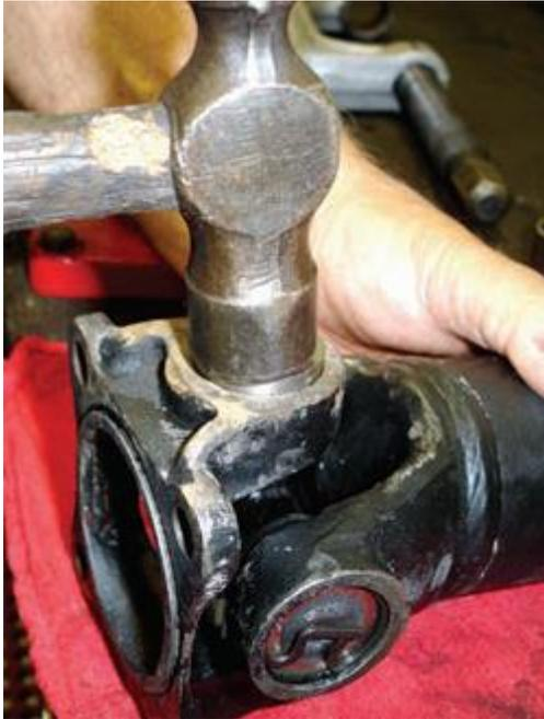
Carefully and precisely use a light-duty hammer to install the U-joint cups. Lift the U-joint up and out of the previously installed cup just enough, so that the one you are installing has the rollers on the U-joint trunnions. This is somewhat tricky so avoid letting the U-joint trunnions drop. If it does drop, it can knock a roller loose.
