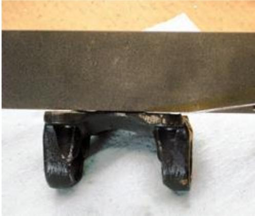
After removing stubborn universal joints, you typically find axle shaft flanges have been distorted. Use a straight-edge to check for distortion. In this case, I found one that is bent. Oh well, it is to be expected when extra force is necessary to remove stubborn U-joints.
