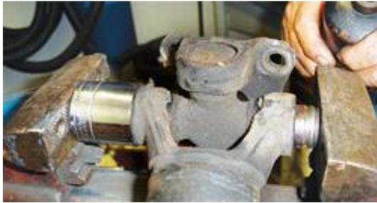
Here's a handy way to replace the U-joints. The chrome socket is large enough to allow the U-joint cup to receive it. Use a smaller-diameter U-joint cup than the one you are removing, so you can apply force and press the U-joint out. If the parts have not been corroded, this often works well. If the cup is old and corroded, it is often frozen in place and this won't work; you may need to use a vise.
