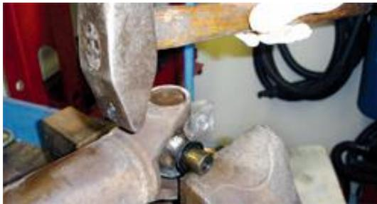
This method also works well, but you must be careful to hit between the weld and yoke flange. The sharp impact of a hammer and tool loosens corroded, stubborn, universal joints. This large hammer works well to get them moving when the vise attempt fails. Be sure to hit squarely at the weld area.
