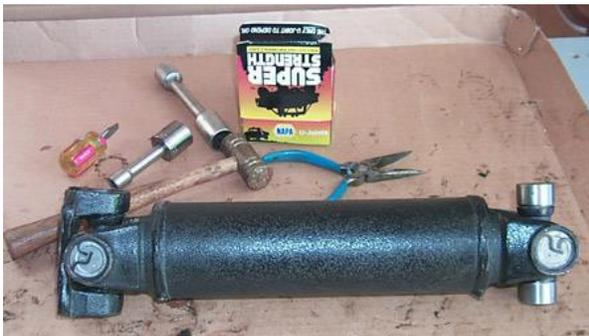
Here's the half-shaft with new u-joints at both ends, ready to go back in the car.
