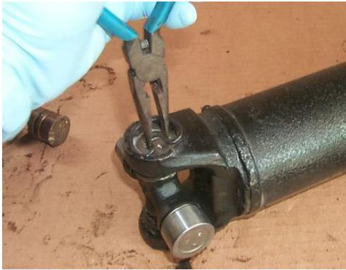
Use needle-nosed pliers to install a snap retainer clip over the bearing cup so that it seats in the groove of the flange.
