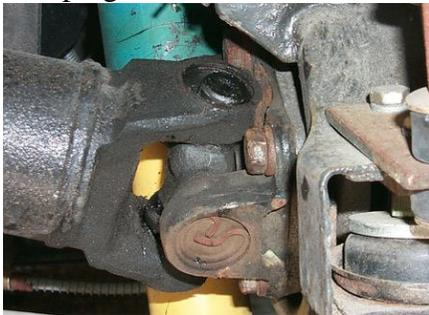
As you can see, the slapping of the u-joint spline against the trunnion made its mark.
