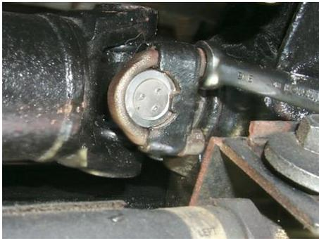
Install the lock washers and nuts on the u-bolts and use a gear wrench to tighten them down. Rotate the tire and re-check tightness of the nuts on both u-bolts, then proceed to install the half-shaft on the opposite side of the car, repeating all of these procedures.
