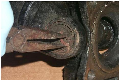
On the workbench, use needle-nosed pliers to remove the snap retainer rings on the u-joints.
