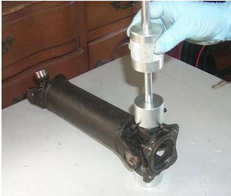
The receiver cup is placed on the lower half of the flange to receive the bearing cup as it is driven out. The hammer with the button installed is placed on the upper bearing cup and the sliding weight raised and slammed down to drive the lower bearing cup out. The half-shaft is then flipped over and the procedure repeated to remove the remaining bearing cup.
