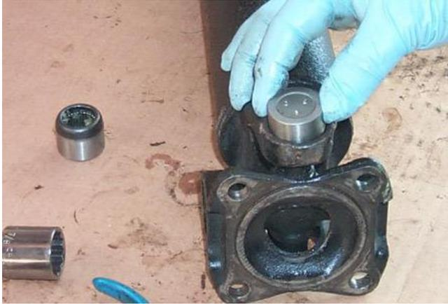
Joining the trunnion with the half-shaft is the next step. Insert the remaining ends of the u-joint (with bearing cups removed) into the half shaft, then place a bearing cup on one end.
