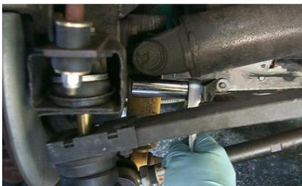
Use a ratchet and socket to remove the four bolts that hold the trunnion (half-shaft flange) to the wheel assembly.
