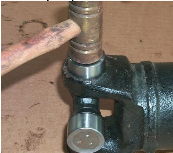
Place a bearing cup on one of the u-joint splines and tap it down with a mallet, then flip it over and repeat the procedure on the other side.
