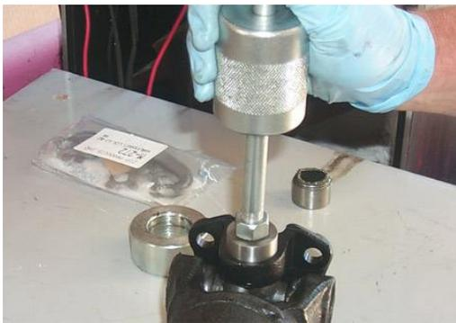
Repeat the installation procedures as before to seat the bearing cups using either the Zip tool or the socket/mallet combo again. Then install the snap retainer clips and make sure they are seated properly.
