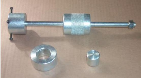
Zip Products also has a special tool available for removing and installing u-joints, shown here. It consists of a sliding cylindrical hammer (top), a receiver cup (lower left) and a button (lower right). The button goes into the lower bout of the sliding hammer and is retained by tightening the four Allen screws for removing u-joints.
