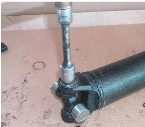
You can use a 7/8 inch socket or the Zip tool to sink the bearing cup down just slightly below the groove that holds the snap retainer clip.
