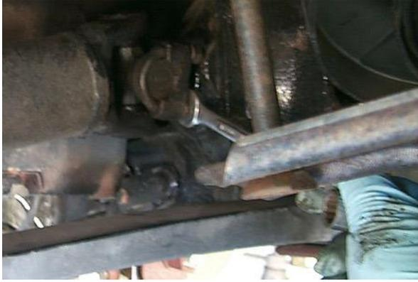
The nuts of the u-bolt that hold the u-joint to the rear differential spline shafts are removed next. A gear wrench definitely makes this task easier, since you'll only have about 7-10° of wrench swing because of the proximity of the struts, spring and stabilizer bar.
