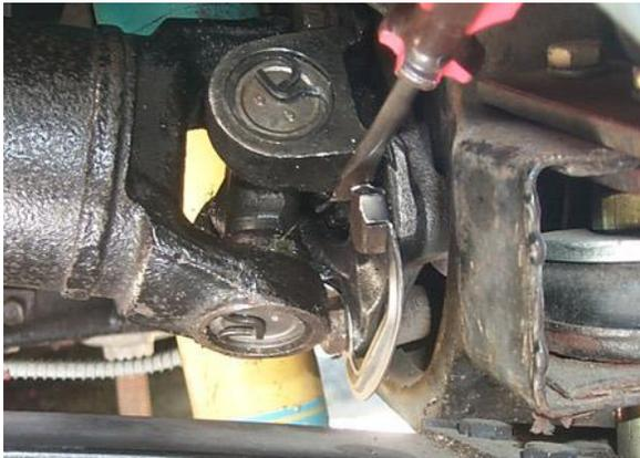
After tightening the trunnion bolts, use a screw driver to bend the ears of the French locks down against the heads of the bolts; this will prevent them from working their way loose.
