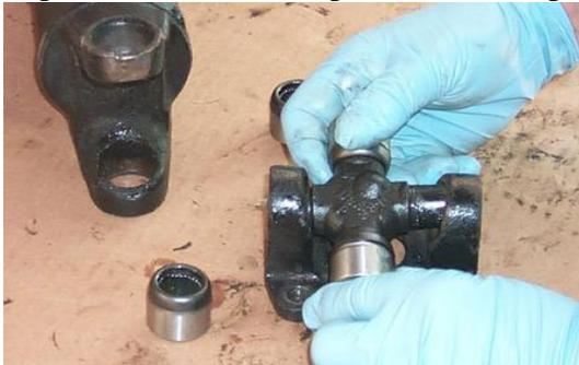
Next, place a new u-joint sans bearing cups in the trunnion, install the bearing cups using either the 7/8 socket/mallet combo or the Zip tool, install the snap retainer clips and tap them home as shown in the previous steps.
