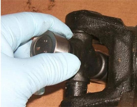
Place a new u-joint with the bearing cups removed in the differential-side flange of the half shaft. Be careful when you remove the bearing cups, as they are lined with needle bearings which can fall out fairly easily.
