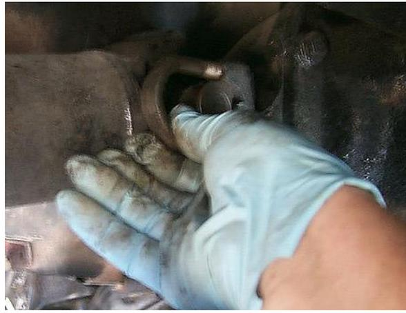
When the nuts are off, remove the u-bolts. You may need to wedge a screw driver between the u-bolt and the u-joint bearing cup to persuade them out. With the u-bolts out, by rotating the tire about half-way in either direction, you'll be able to slide the entire half-shaft with u-joints out.
