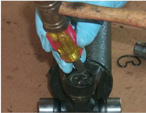
Use a screwdriver and mallet to tap the snap retainer clip all the way into groove; this is very important, since this clip can and will spring out if it isn't solidly seated in the groove.
