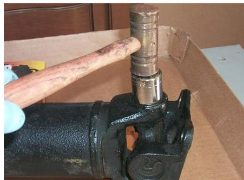
Support the half-shaft with a block of wood so the lower bearing cup is elevated from the work surface. Use a 7/8 inch socket and mallet to tap the upper bearing cup down, which will drive the lower cup out of the half-shaft. After removing the lower cup (a pair of vice-grip pliers may make it a bit easier to extract it if it's stubborn), flip the half-shaft over and repeat the process for the remaining bearing cup.
