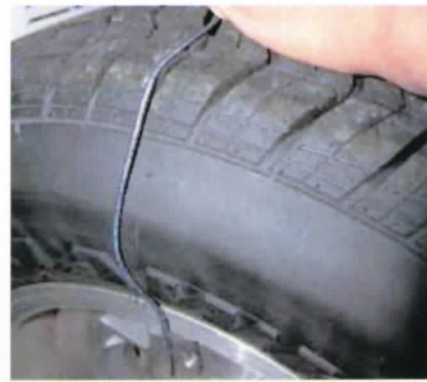
Bend the wire over an existing tire to obtain a rough initial shape.
