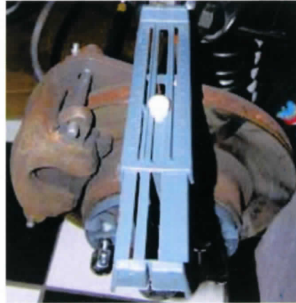
Adjust the WheelRite to the width and height of the desired wheel and attach it to the hub.
