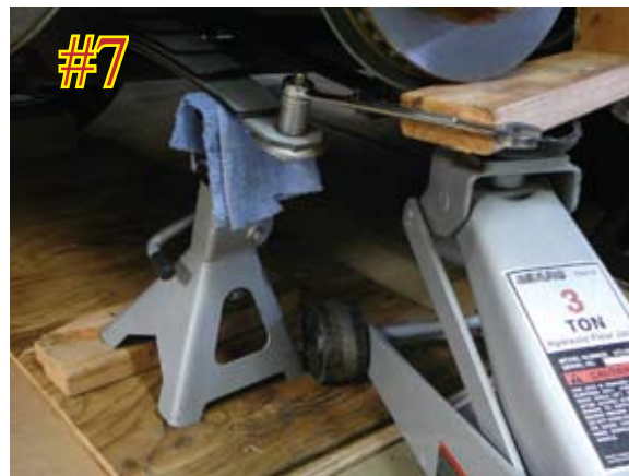
#7 Photo showing the swaging tooling in place to perform step one of the swaging process for the retainer cup at the end of the leaf spring. The entire swaging process of all four retainer cups can easily be done by one person in a few hours.
