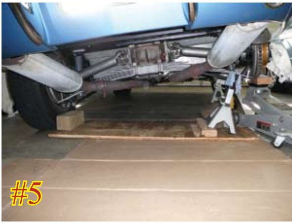
#5 Plywood and blocking system in position to allow removal and replacement of the retainer cups on the passenger's side. The sequence of steps leading up to the stage shown in this figure is explained in detail in the text.
