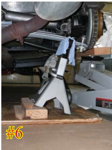
#6 Close-up photo showing the position of the jack stand under the end of the leaf spring. Note that the vertical axis of the jack stand is close to perpendicular to the arch of the spring. This photo shows the stage of the process after removal of the link bolt, with the new retainer cup in place and with the swaging tooling in place ready to perform the swaging step.
