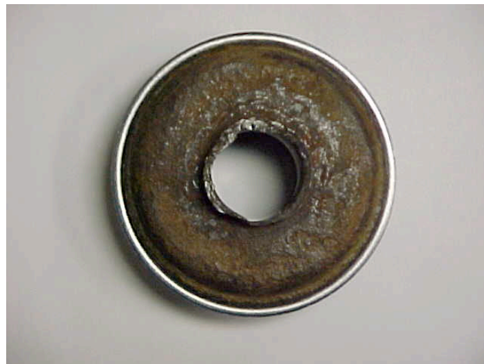
Fig. 4 Top view looking down onto a rusty original retainer placed face to face against a newly modified retainer showing a slight increase in the radius of the peripheral lip on the modified part.
