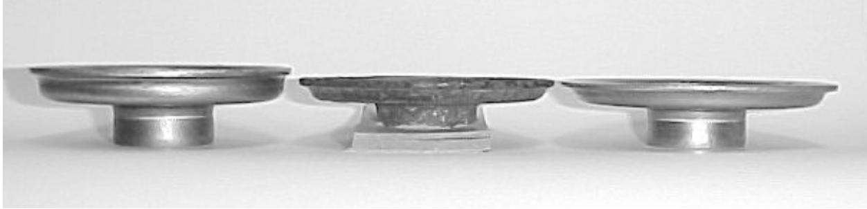
Fig. 3 Photo showing the currently available GM retainer (left), an original retainer (minus a portion of the bottom section that was destroyed during removal) from an original 1966 leaf spring, and the modified retainer (right) that more closely approximates the lip height and angle of the original mid-year retainers.
