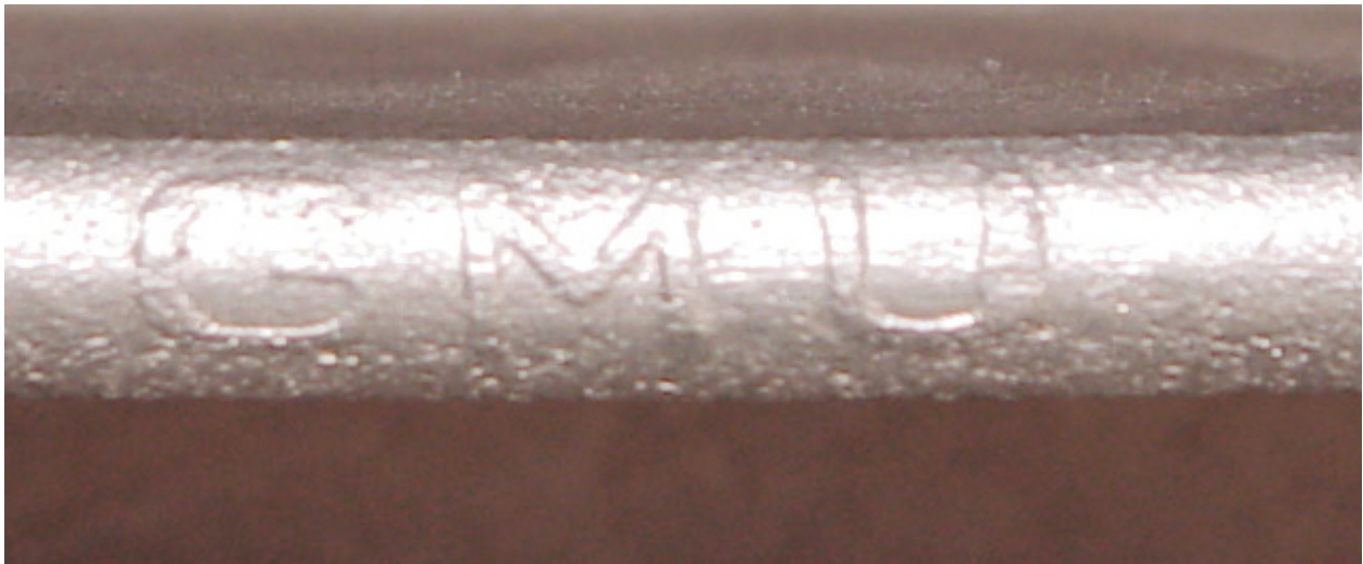
Fig. 1 Photo of "GMU" embossing on a 7-leaf, heavy duty spring (photo by Craig Schultz). This embossing has also been observed on 9-leaf, standard springs.
